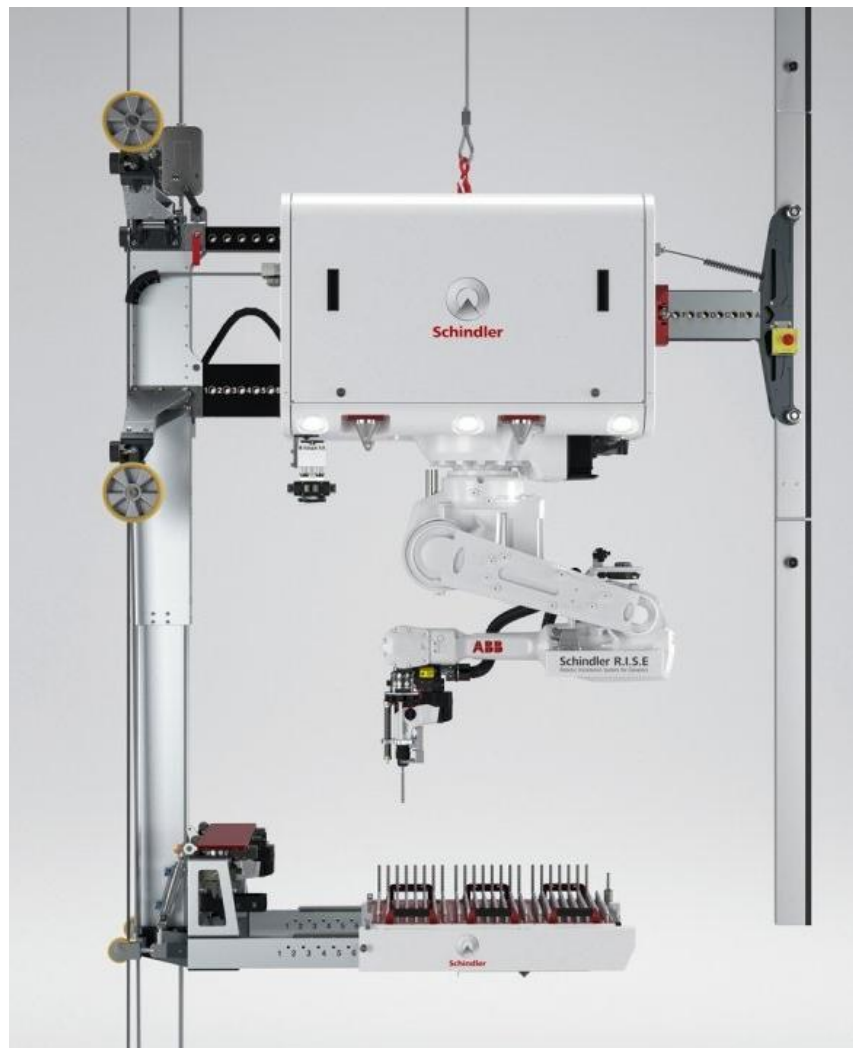
Figura 9.5-3. Fotografía del Robot RISE (Robotic Installation System for Elevators)
